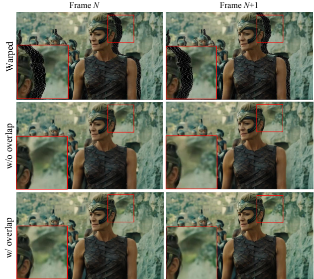
Figure 9. Ablation results of auto-regressive modeling. We concatenate the last n frames generated from the previous round with the warped frames of current round as input. When n = 0 , i.e., without overlap, the inpainting results of adjacent rounds cannot maintain temporal consistency, as shown in the second row.
